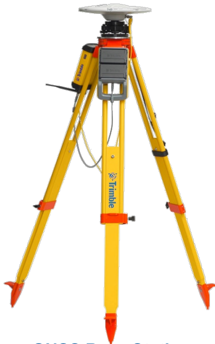
GNSS Base Station
